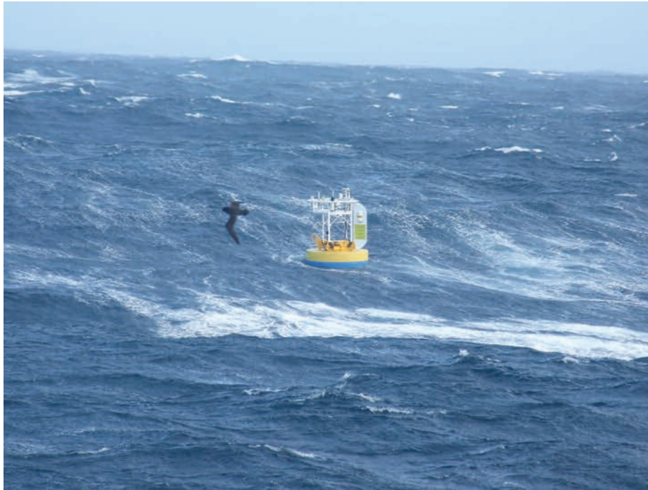
Figure 32: Air-sea flux mooring deployed at 47°S, 140°E south of Tasmania as part of Australia's Integrated Marine Observing System (IMOS). This is the first air-sea flux mooring so far deployed in the Southern Ocean and will be used to assess the quality of air-sea flux products derived from satellites and reanalysis products. Courtesy of Eric Schultz, Australian Bureau of Meteorology.
